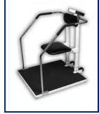
extra wide platform adds comfort to the weighing of obese patients and those requiring assistance. The 6868 tips back for easy transporting. The large diameter wheels and handrail make it easy to move from place to place. The compact design permits the scale to fit through doors and into patients' rooms for easy weighing (requires door opening greater than 32" / 813mm wide).
