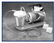
replacing the cap and float assembly with a hydrophobic bacteria filter. This filter prevents fluids and other contaminants from damaging the pump. This durable unit continues to meet the need for controlled vacuum regulation from 0-22" Hg with a flow rate of 28 lpm. Weighs 13.6 pounds, 1/15 hp motor, 115V, 60 Hz.
