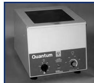
Performs centrifugal blood cell separations, urine separations, and sperm cell washing. Offers the larger laboratory or hospital these important features: 24 place angle head, variable speed (calibrated in both RPM and RCF), and automatic braking system. 3 Year Warranty.
