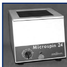
Offers reliable microhematocrit determinations. The high speed motor assures rapid spin-downs, and the included reader is adjustable, allowing accurate readings in a variety of circumstances. Quieter operation than many similar units, the Microspin offers
